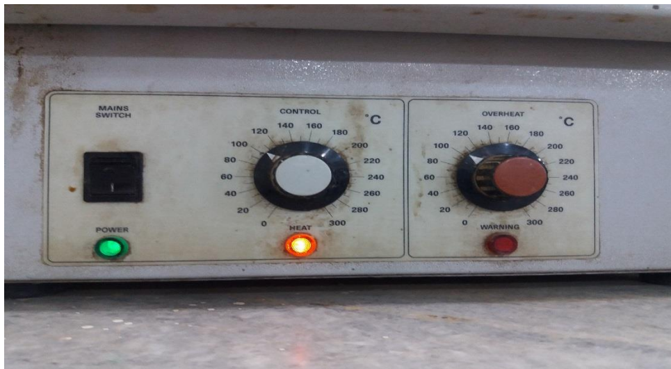
Figure (3.7) shows evaporation furnace.
