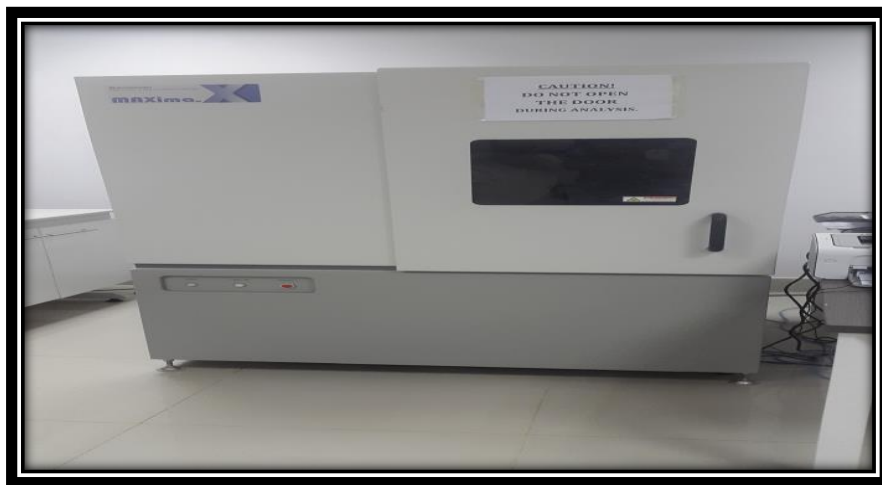
Figure (3.6) X-Ray diffract meter: XRD (wavelength 1.54 \text{ \AA} )
