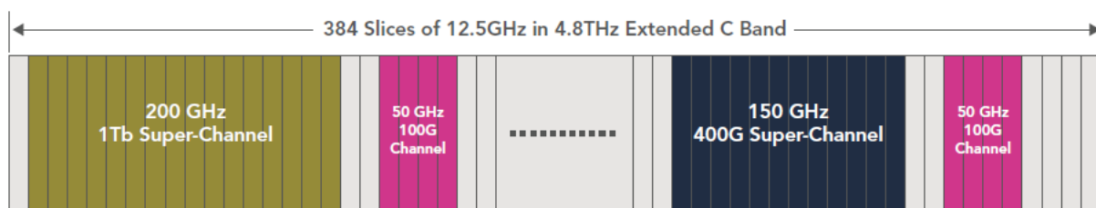
Figure 2.5 ITU-T G.694.1 Flexible Grid Architecture
