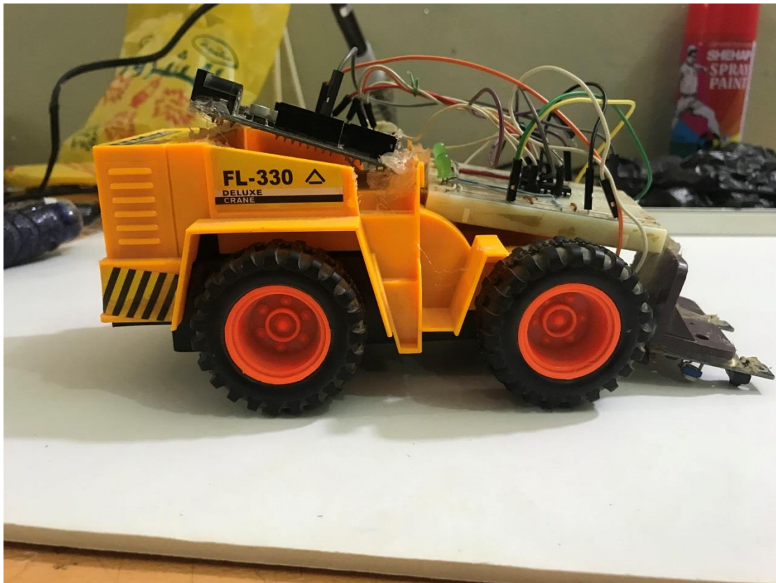
figure (4.1) Side view of bread board and Arduino connected up to the car
