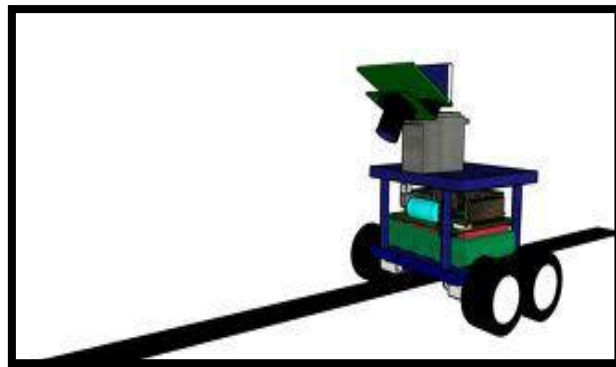
Figure (2.3) LFRV Using LDR And LED Sensor
