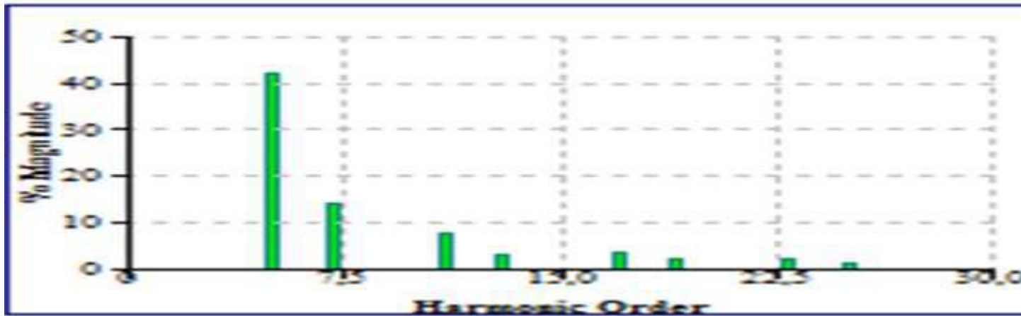
Figure 3.8: Harmonic Source Spectrum for VFD
