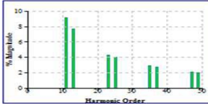
Figure 3.10 : Harmonic Source Spectrum for UPS
