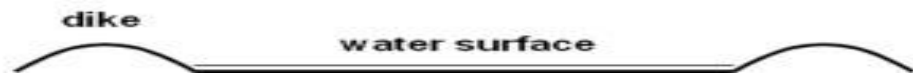
Figure 2.2: Schematic of a border-irrigated field, where a uniform sheet of water flows between dikes.
