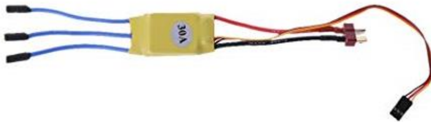
Figure 3.19: 30A Electronic speed controller
