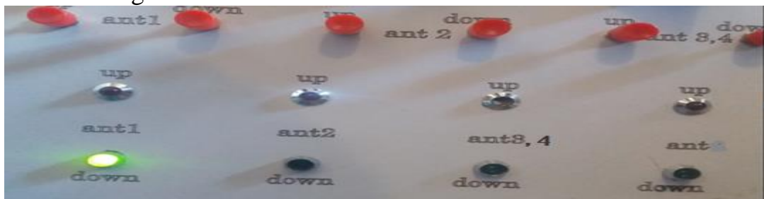
Figure 4.50 Indicator of Antenna1 Moves to Dawn Position
