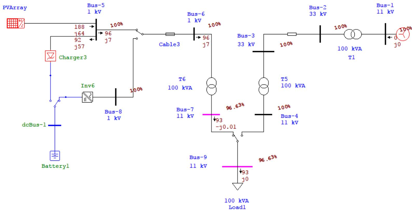
Figure 4.11: Case two's load flow analysis
