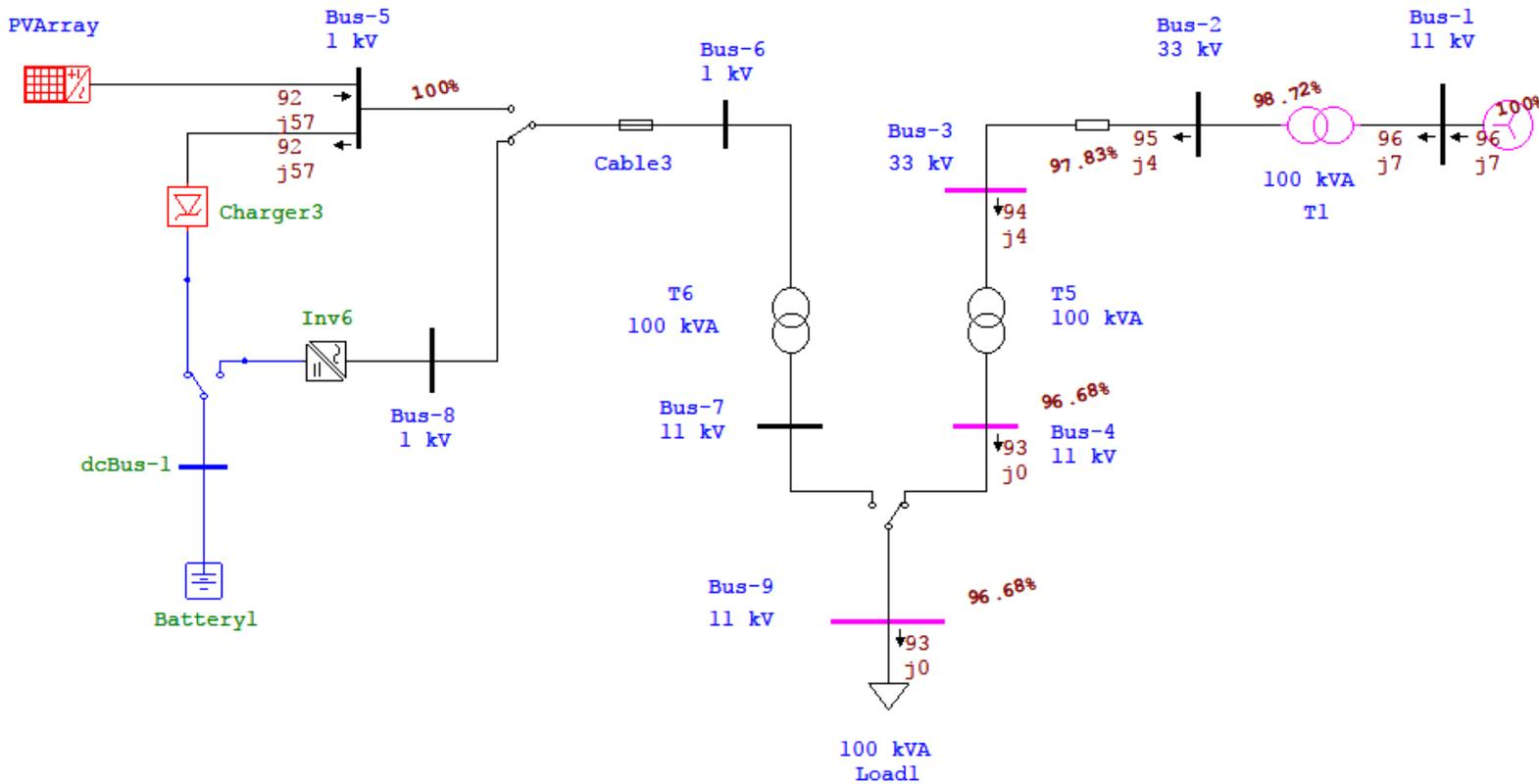
Figure 4.13: Case four's load flow analysis
