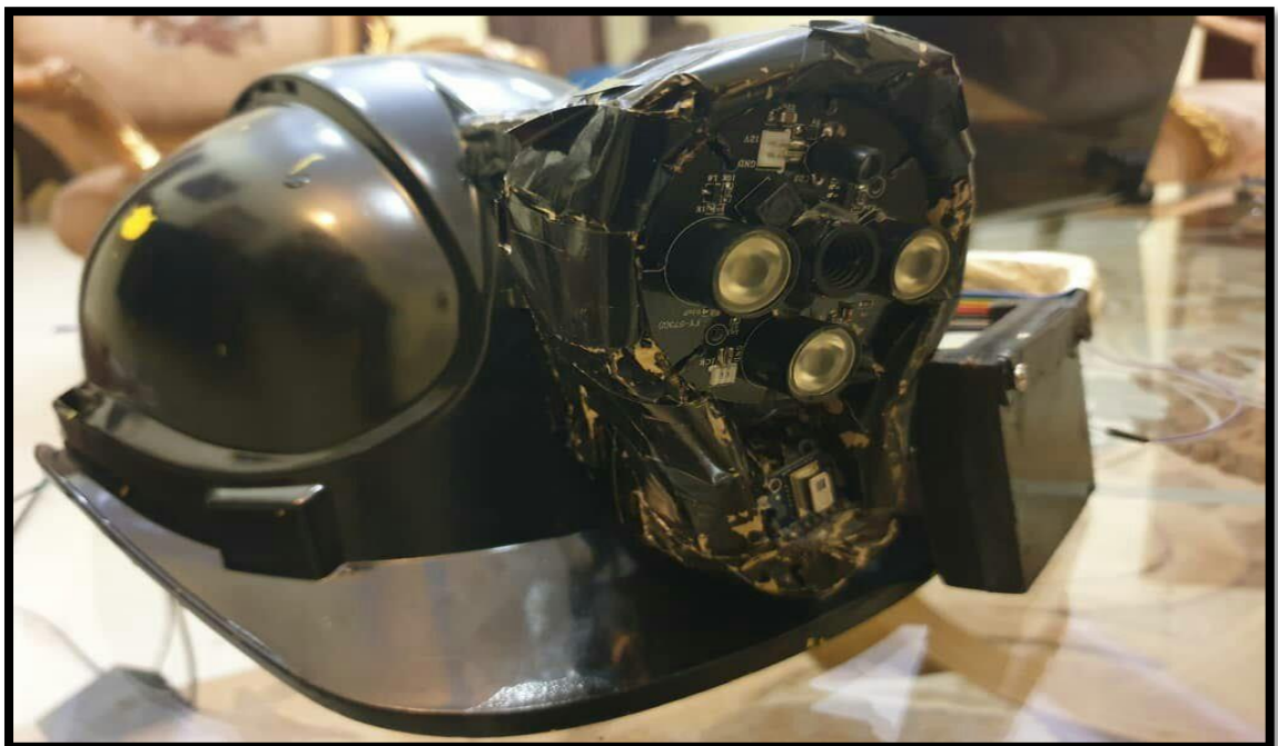
Figure 4.6: Night and thermal camera attachment.
