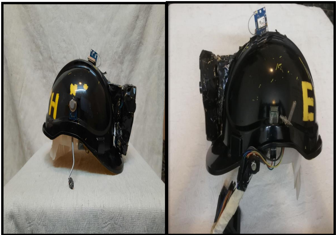
Figure 4.8: Communications modules, sensors and GPS fixing
