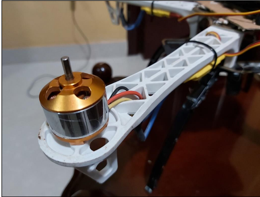
Figure 4.4: Brushless DC Motor Screwed on Quadcopter Arm.
