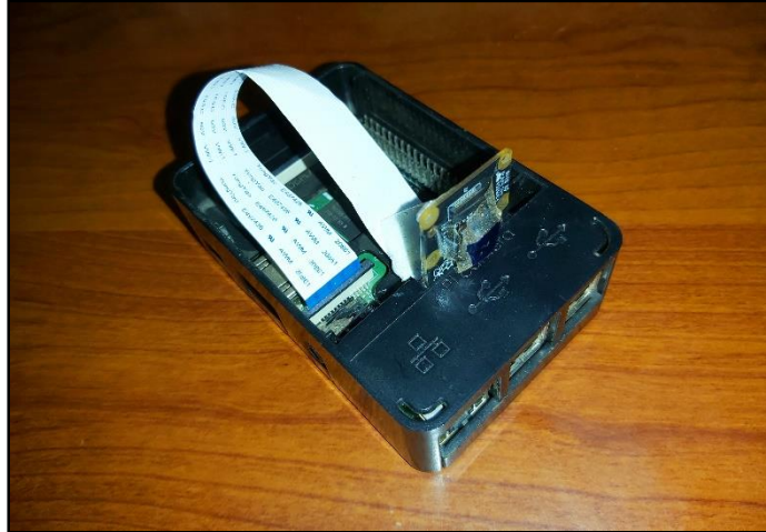
Figure 4.21: Connection NOIR Camera to Raspberry Pi 3 CAM Port.
