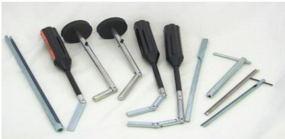
Figure 2.8 : Hoistway Door Emergency Keys
