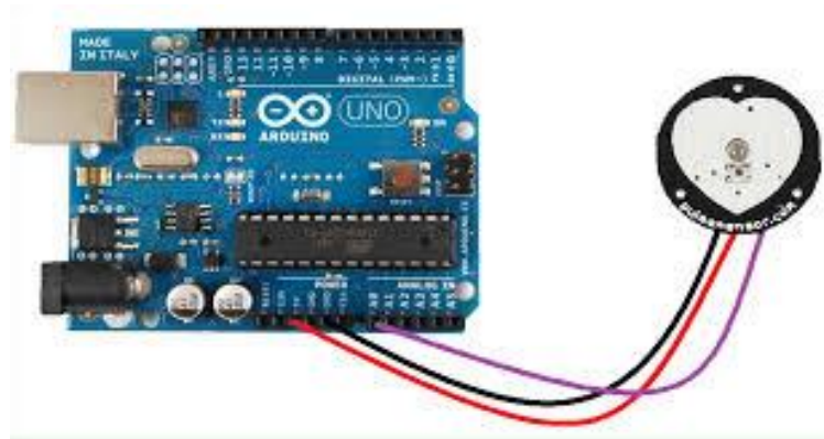
Figure 3.8: Interfacing Arduino with heartbeat sensor
