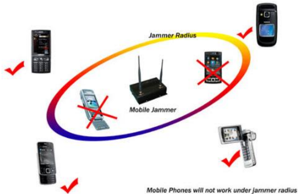
Figure 2.1: Mobile jammer and jammer radius
