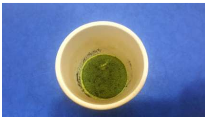
Photo (4.1) Sample mixture of chromites ore, sodium carbonate, and calcium carbonate after heating
