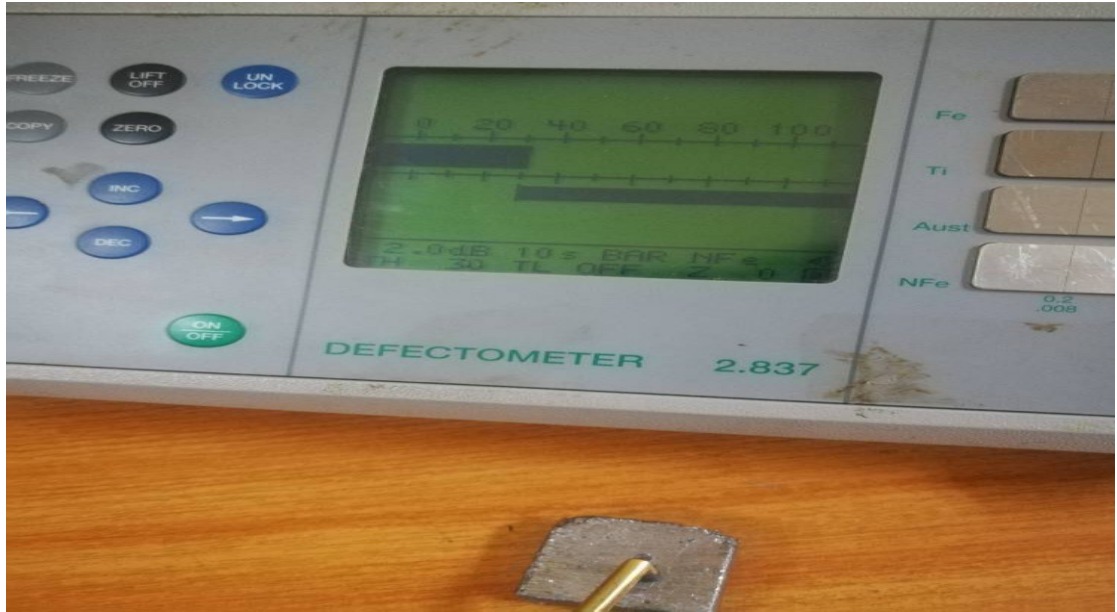
Figure (4.3) shows Pb samples inspected with defect 30%
