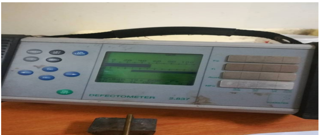
Figure (4. 10) shows Fe sample with defect 50%
