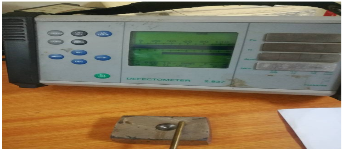
Figure (4.6) shows Tutia sample inspected with defect 100%
