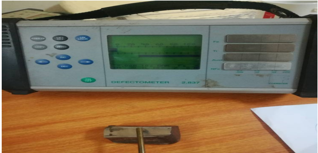
Figure (4.5) shows Fe sample inspected with defect zero
