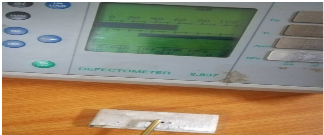
Figure (4.4) shows Al sample inspected with defect 60%
