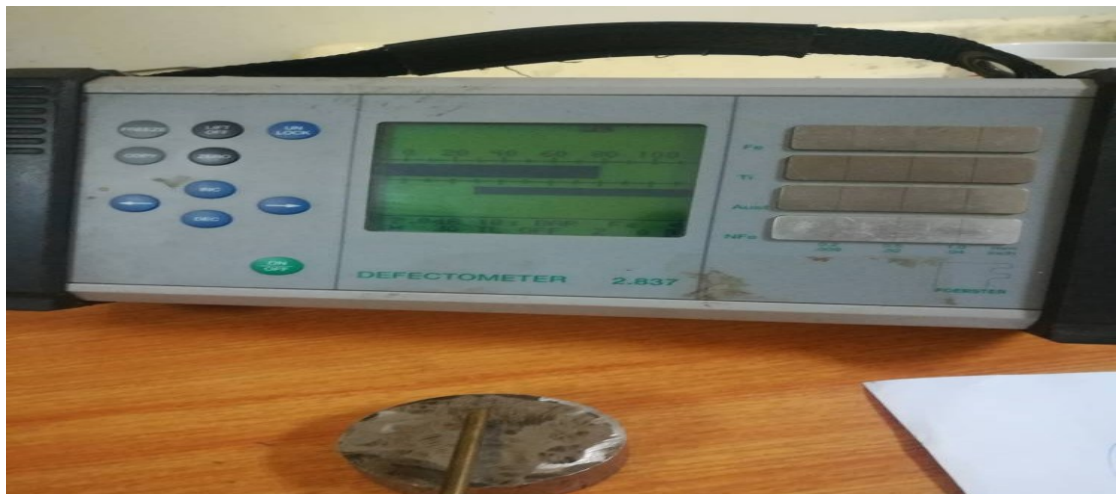
Figure (4.7) shows steel sample inspected with defect 80%
