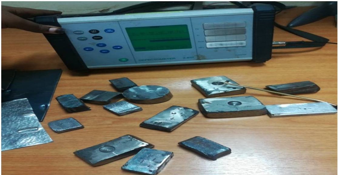
Figure (4.2) shows the Defect meter 2.837 with samples to be inspected
