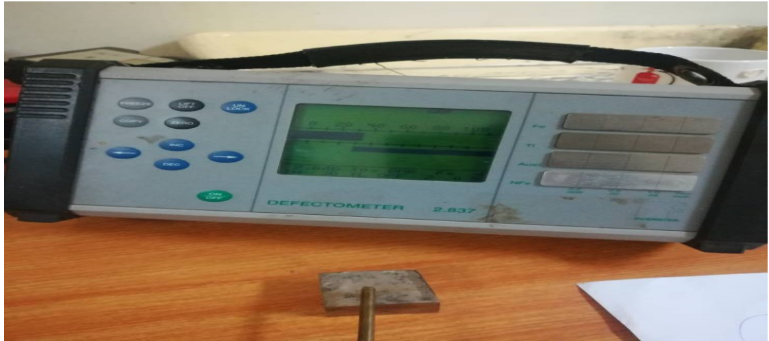
Figure (4.11) shows steel sample defect 30%
