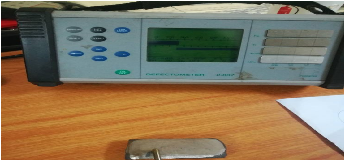
Figure (4.8) steel sample inspected with defect 30%
