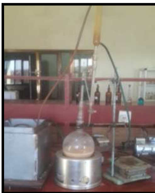
Figure (3.4): Soxhlet Extraction
