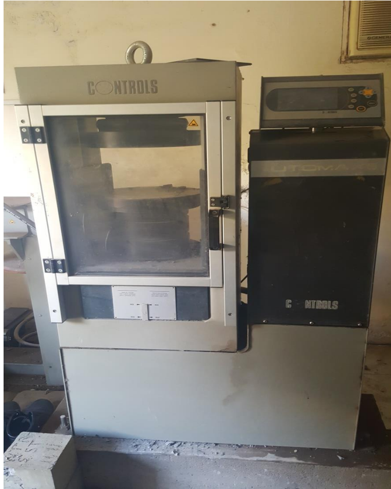
Figure (3.3): MATEST C104 Servo Plus 2000 KN Capacity Compression Test Machine .
