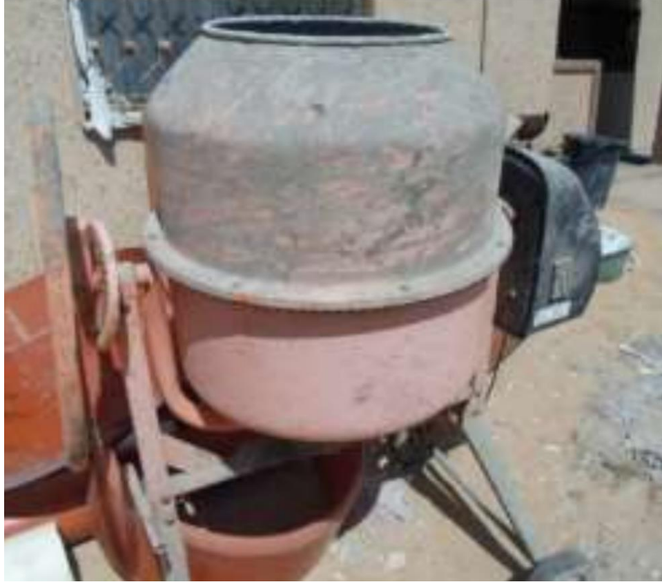
Figure (3.1): The Power-Driven Revolving Drum Mixer Used on This Research.
