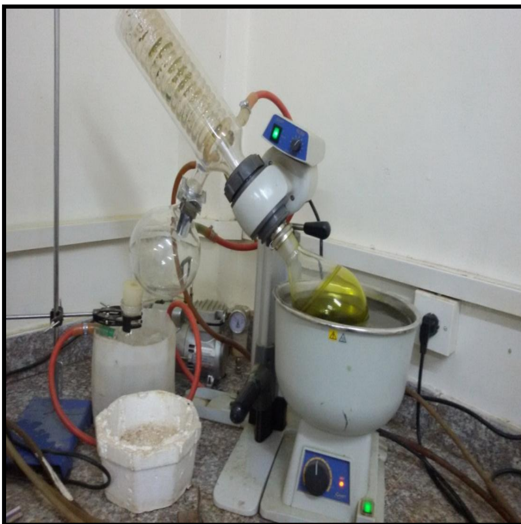
Plate 7. Vacuum Rotary Evaporator for separation of solvents.
