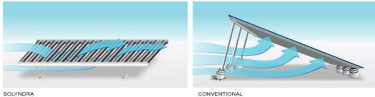
Fig. [2.8] : Wind effect on solar panels .
