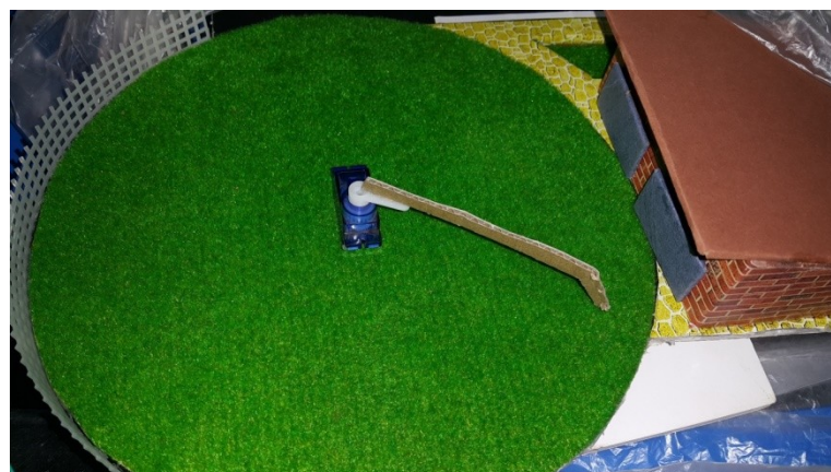
Figure 4.15 : Servo motor acting as pivot irrigation
