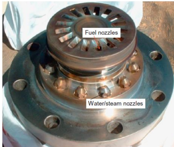
Figure 2.16A typical fuel nozzle showing both water and fuel nozzles for a typical wet diffusion combustor used for NO_x reduction ( NO_x _ 25 ppm).
