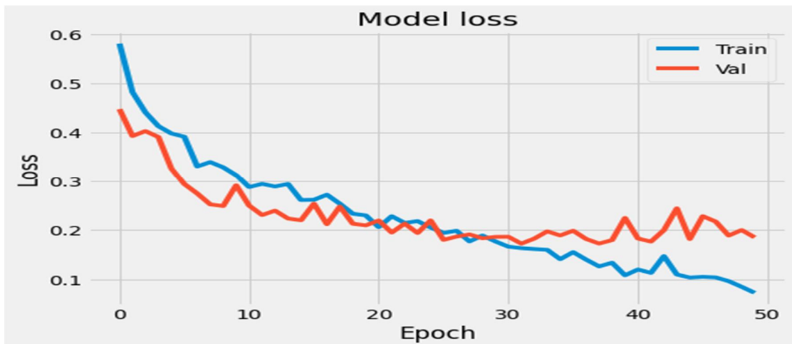
Figure 5.7: plot shows loss for training and validation for 50 epochs without use of cross validation
