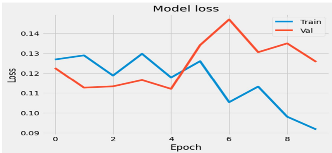
Figure 5.12: Plot shows loss for training and validation for last 10 epochs with use of 5 fold cross validation
