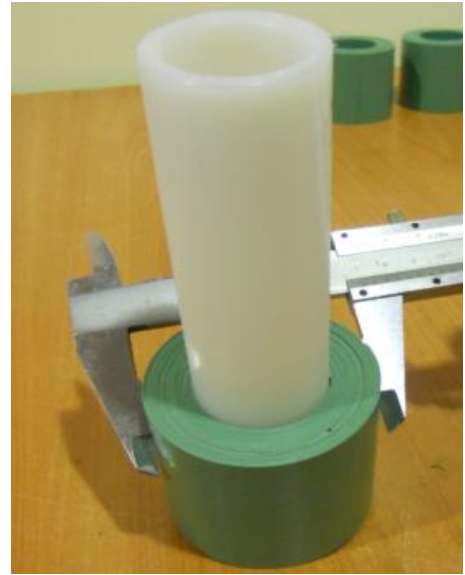
Measure the outer diameter
