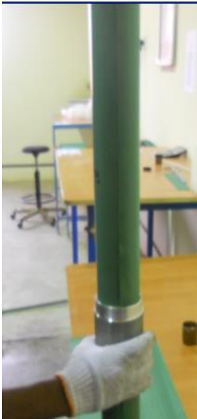
Put the pieces in copper mandrel
