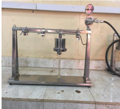
Figure A.7: ZNS-4 Inflator air supply water Loss meter.
