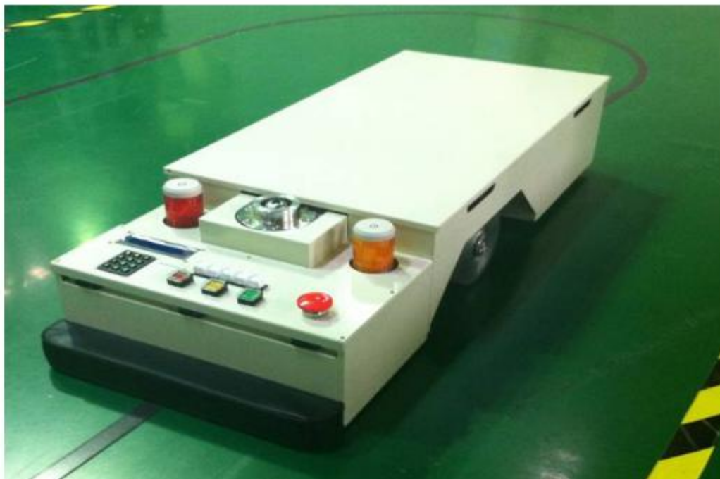
Figure (2.4): An AGV following a magnetic strip [23].
