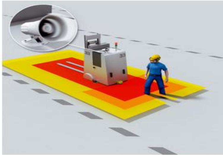
Figure (2.8) : Safety fields for an AGV [24].
