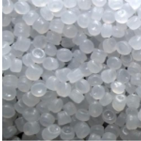
Fig (3,1) LDPE in the form of grain
