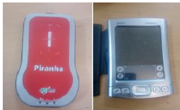
Figure 3.2 Semiconductor detector (Piranha) and display unit (palm)
