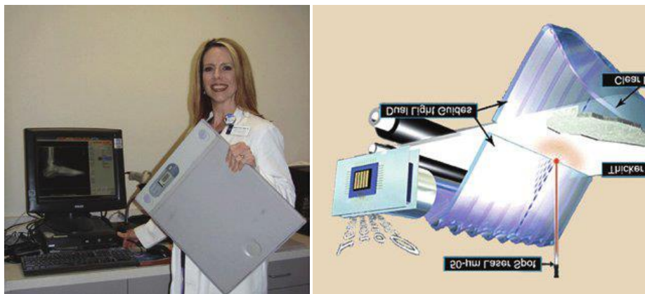
Figure (2.3) shows the computed radiography imaging plate prepared or insertion into electronic reader. (Bushong, 2017)
