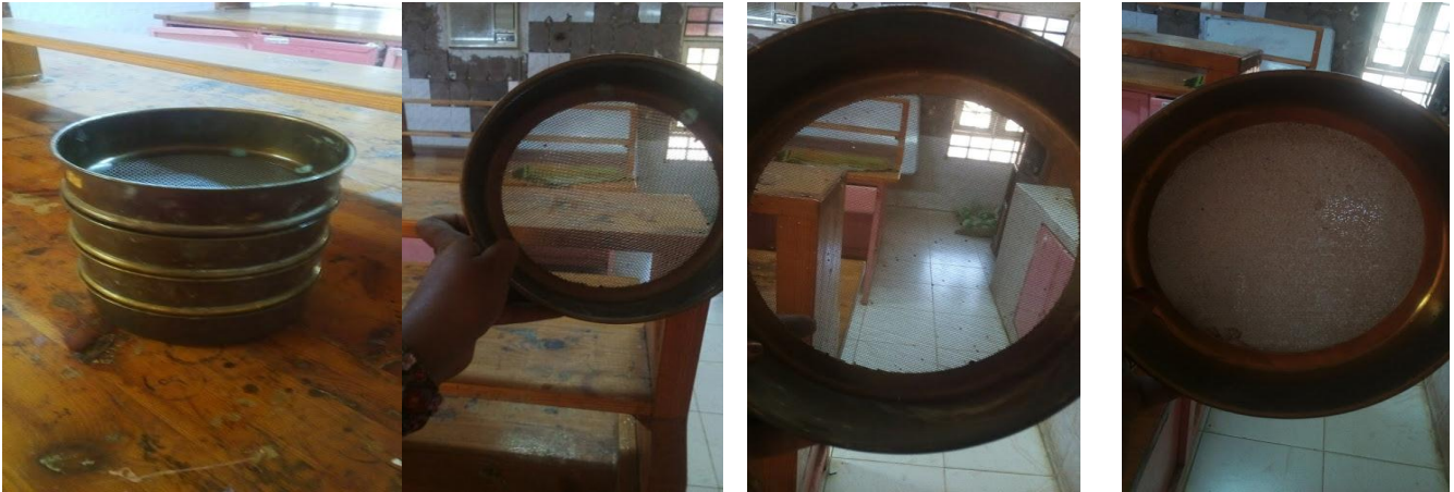
The sieves were used in washed soils – three types of pore size
