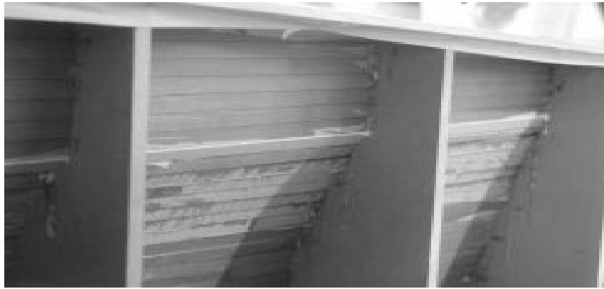
Figure 4-6, One-Off Female Mold (Eric Greene Associates, 1999)
