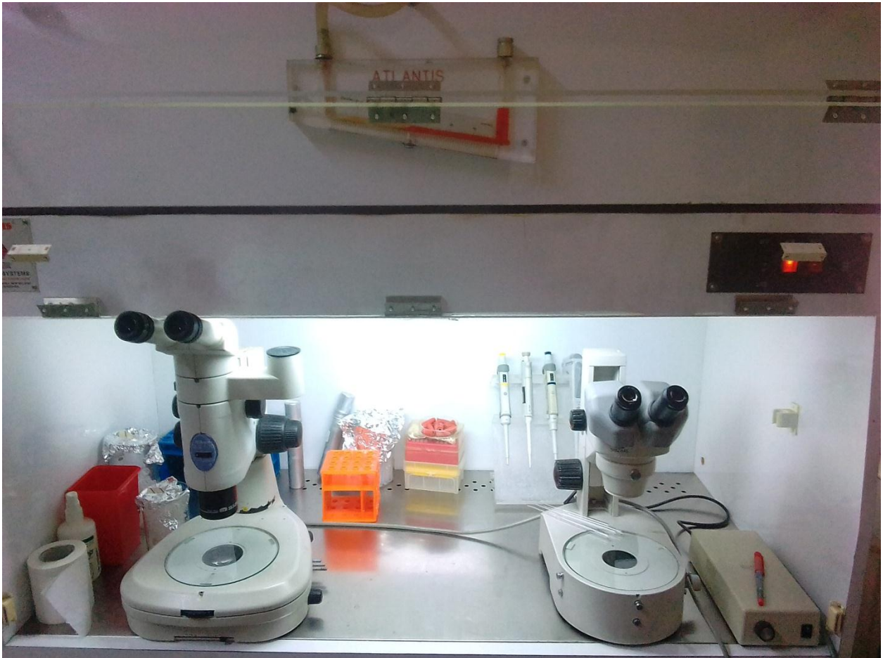
Laminar for searching oocytes, IVM, IVF, IVC and embryo evaluation. Consisting of: 2- stereozoom microscopes, racks, tissue pipettes , tips , glass , mark pen and disinfection spray.
