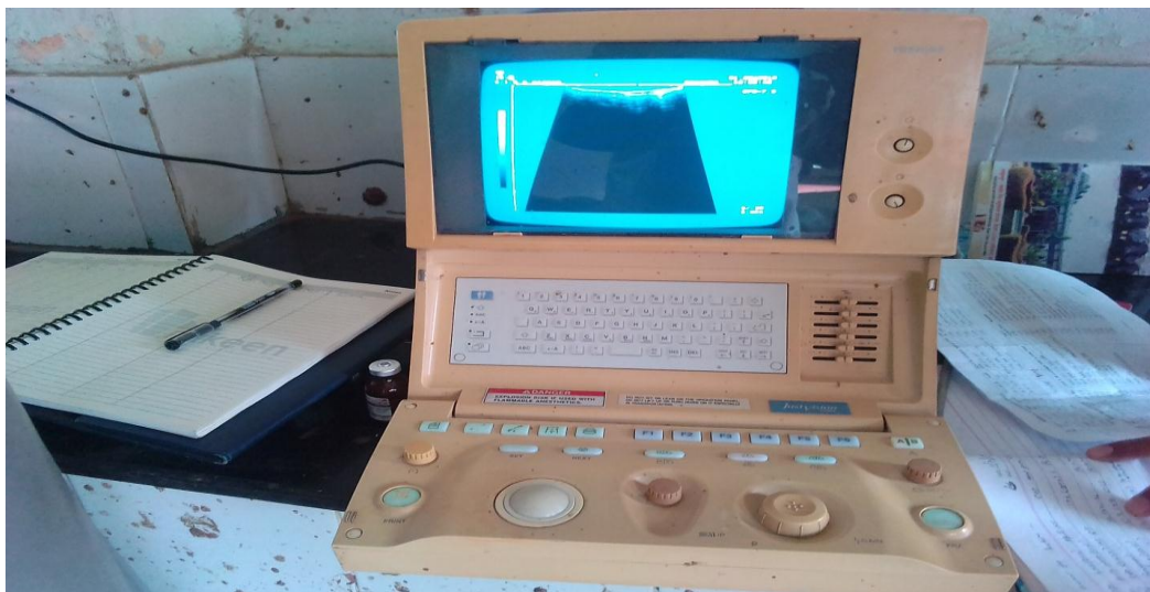
Fig 16: Real-time B-mode trans-rectal ultrasound scanner with an intraoperative 7.0 MHz micro convex transducer.
