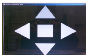
Fig.3-17: 2-Dimensional cursor control where the target detection tasks are presented in four compass positions (N, E, S, W) on a computer screen (Polikoff J., 1995).
