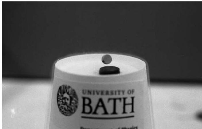
Fig (2.5) Levitation, induced by the persistent surface current and the Meissner effect, of a powerful, small samarium–cobalt permanent magnet above a YBCO polycrystalline sample produced by students in the Department of Physics of the University of Bath.
