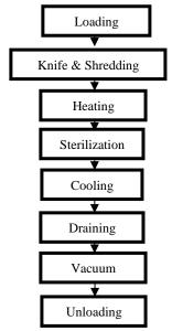
Figure 1: Autoclaving Process flowchart
