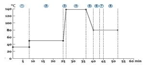
Figure 3: Sterilization Cycle
