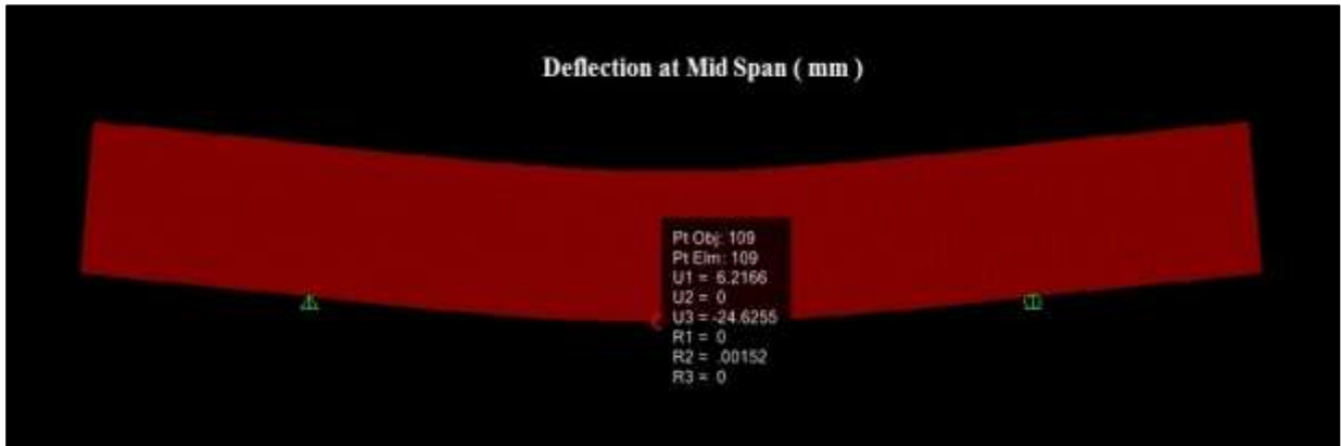
Figure A. 43: Deflection at Mid Span for Beam MS3-2
