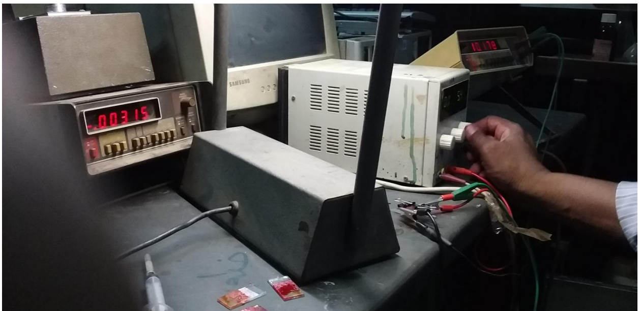
Figure 4.10 Reading (I, V) for solar cell with Bengal rose The samples ready for characterization
