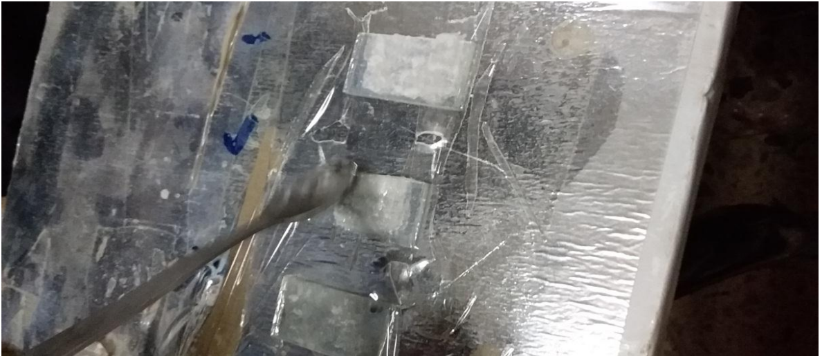
Figure 4.4 Deposition of ZnO nanoparticles onto FTO glass
