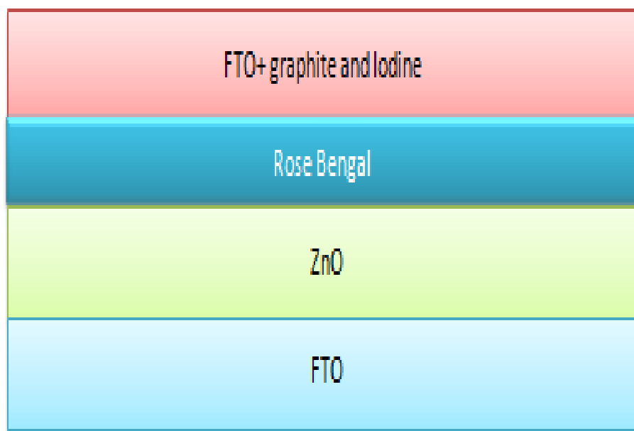
Fig 4.8 schematic structure of (FTO/ ZnO/ Rose Bengal /FTO+ graphite and Iodine)
