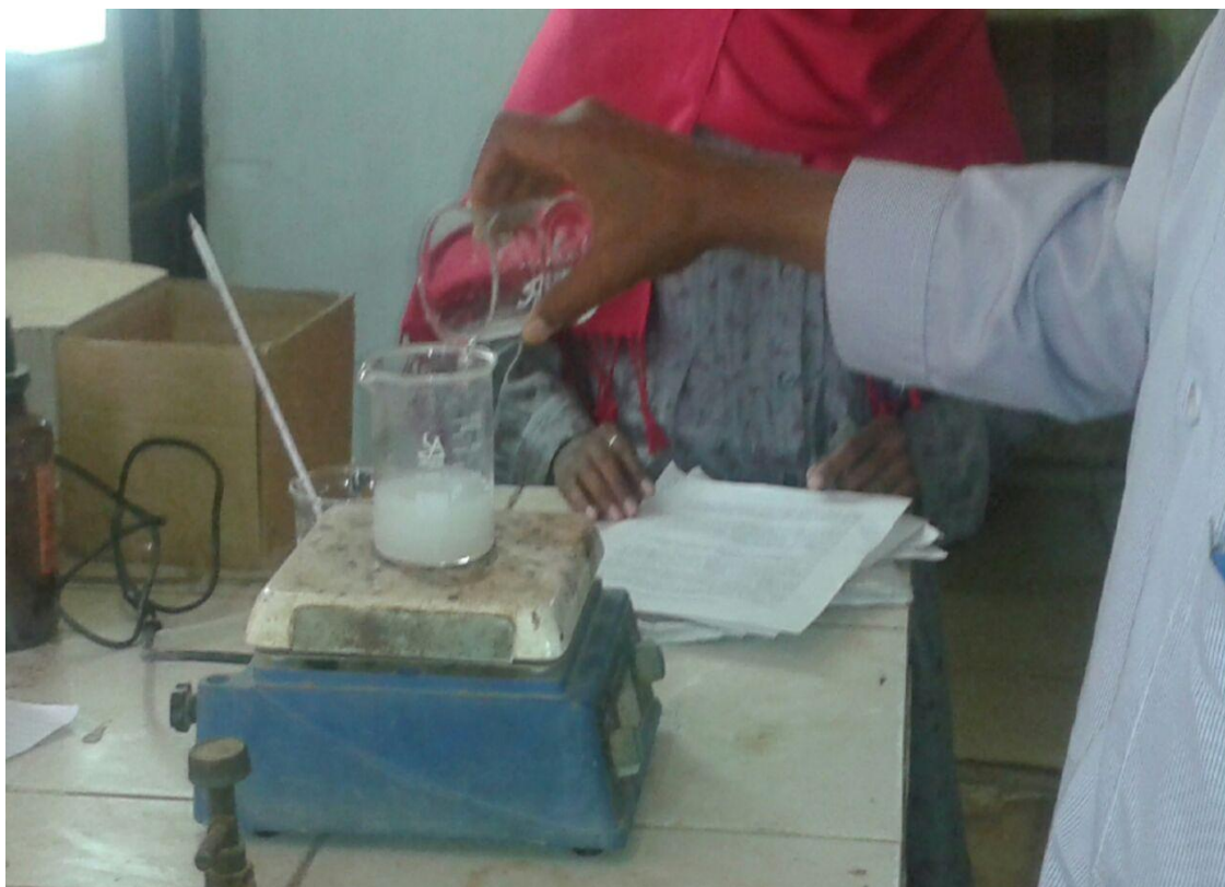
Figure 4.1 heat the solution to 60°C under continuous stirring
