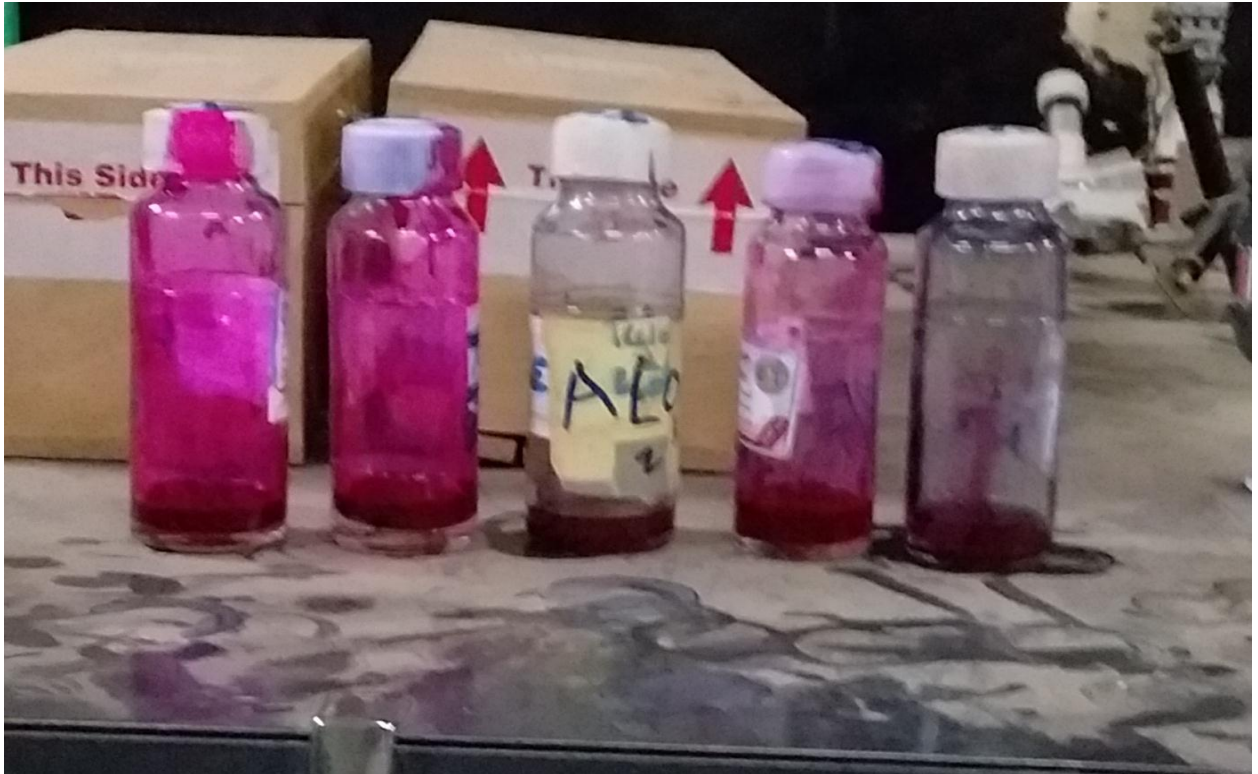
Figure 4.9 Bengal rose dye with (Methanol, Ethanol, Acton, Chloroform and Benzene)
