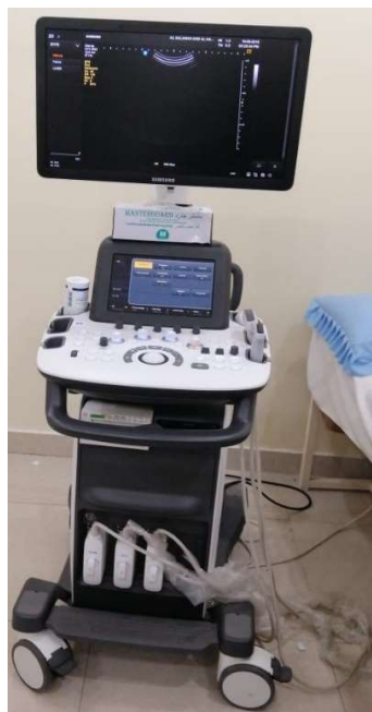
Figure: 3-3-The Samsung UGEO H60. The Samsung UGEO H60 is a high-performance midrange ultrasound machine designed from the ground up by Samsung. Previously known as the UGEO H60, this system features productivity enhancements a touchscreen, large LCD monitor and 4 active probe ports
