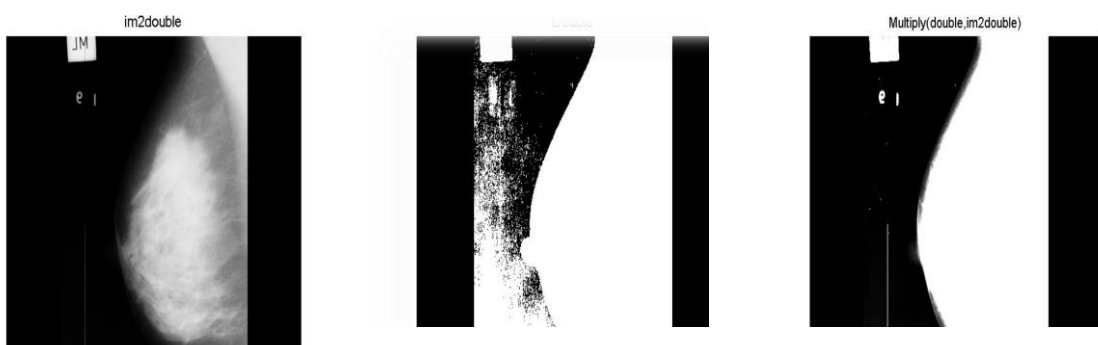
Figure (5-5): Median filtering used for preprocessing: (from left to right ) original image, binary image with noises, and binary image after filtering
