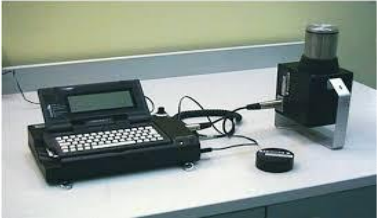
Figure (3.1) NaI (TL) detector based gamma ray Spectrometer
