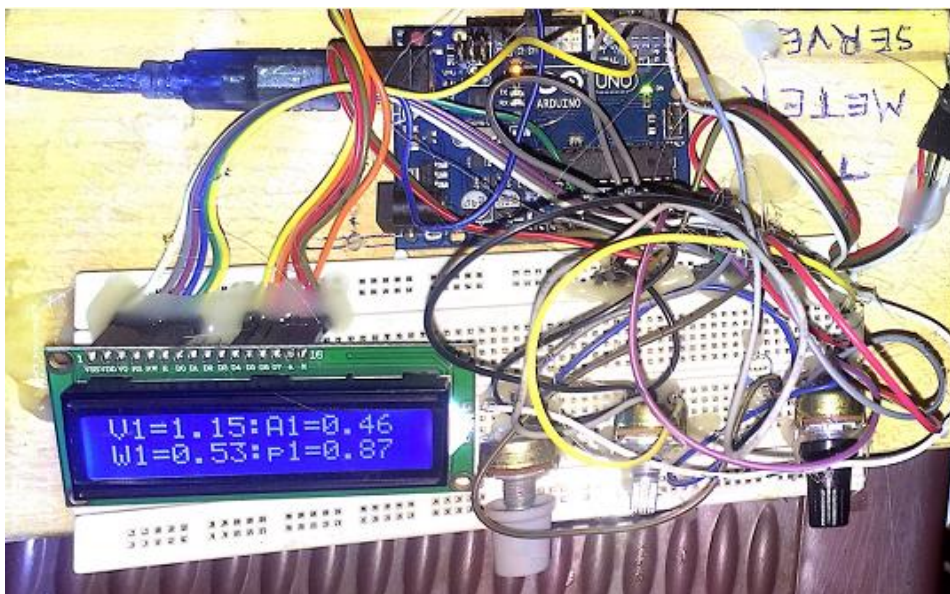
Figure 4-5 watt meter No.1 measured values in the transmitter side
