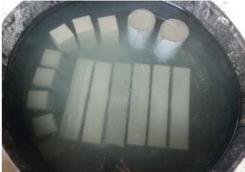
Figure 3.8: Cubes at curing basin
