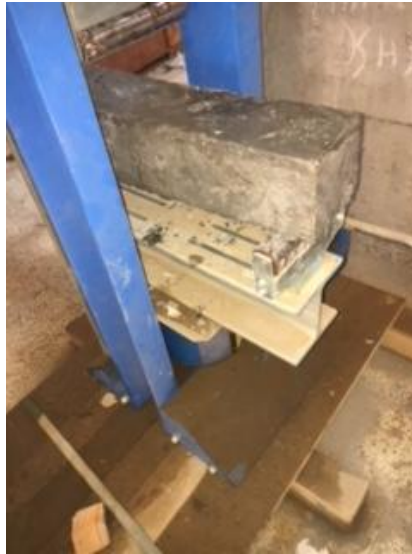
Figure 3.11: Flexural test specimens (100*100*500mm)
