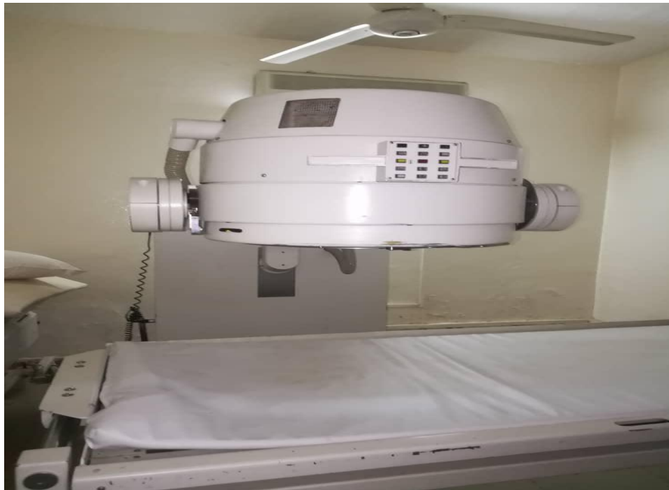
Fig 3.11 Typical SPECT gamma camera (orbital37) installed in Al Nilien Nuclear Medicine Department.
