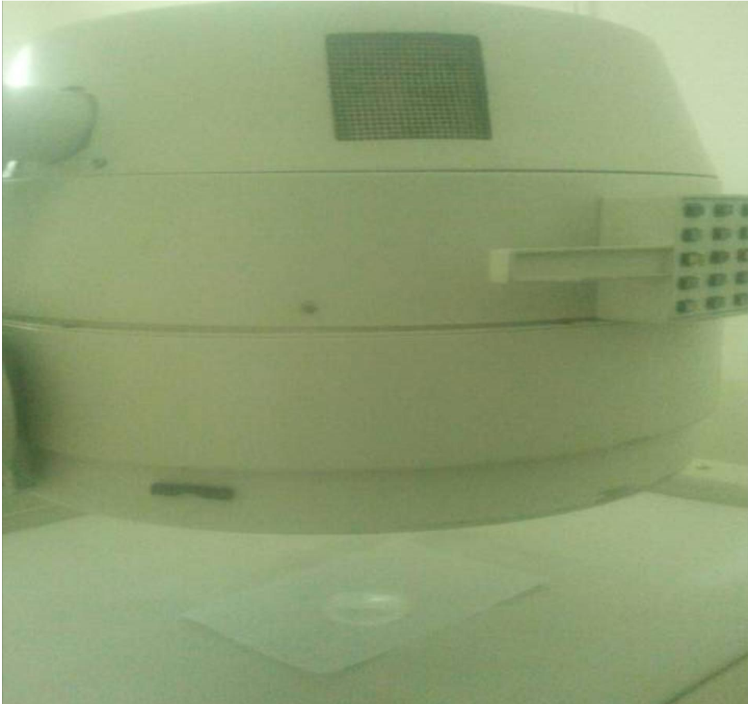
Fig 3.2.4 the position of the plastic dish in the detector center during sensitivity measurement
