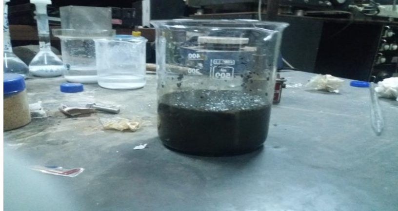
Figure (3.6.a) shows the process of mixing sodium sulfide and silver nitrate
