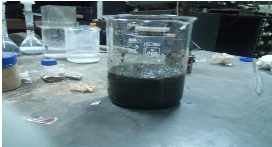
Figure (3.6.b) shows the process of mixing sodium sulfide and silver nitrate
