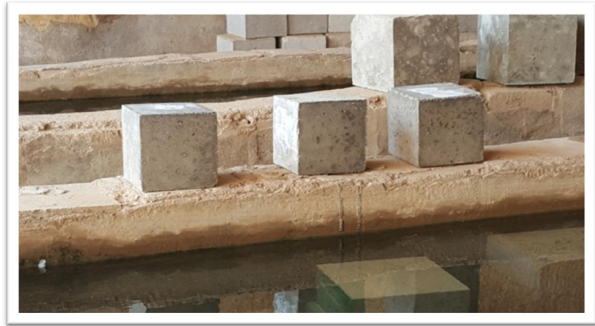
Curing of cubes
