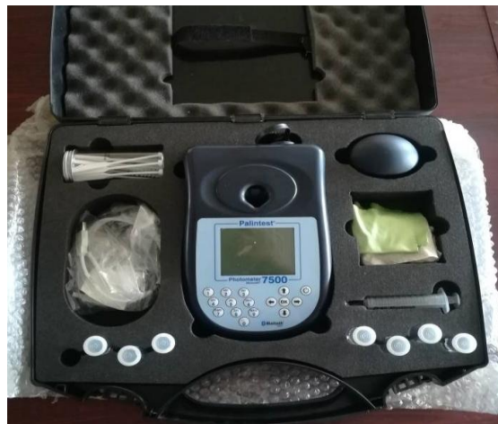
Figure 3.3: Palintest photometer apparatus.
