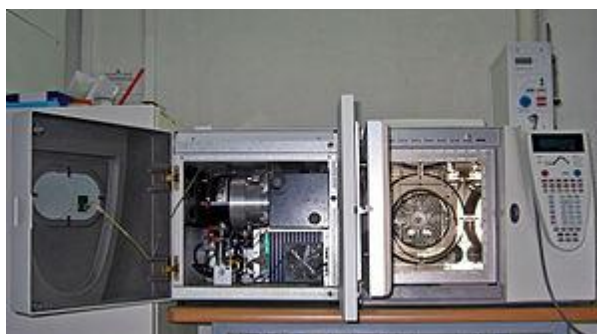
GC-MS instrument - column of the gas chromatograph in the oven on the right
