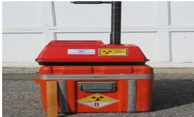
Figure1.4: A portable nuclear gauge
