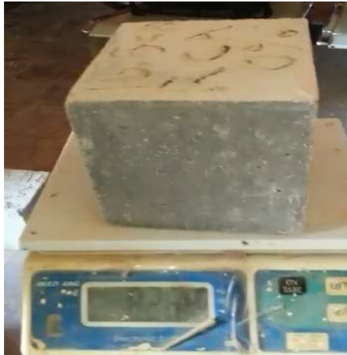
C1 Weight of the cube before crushing
