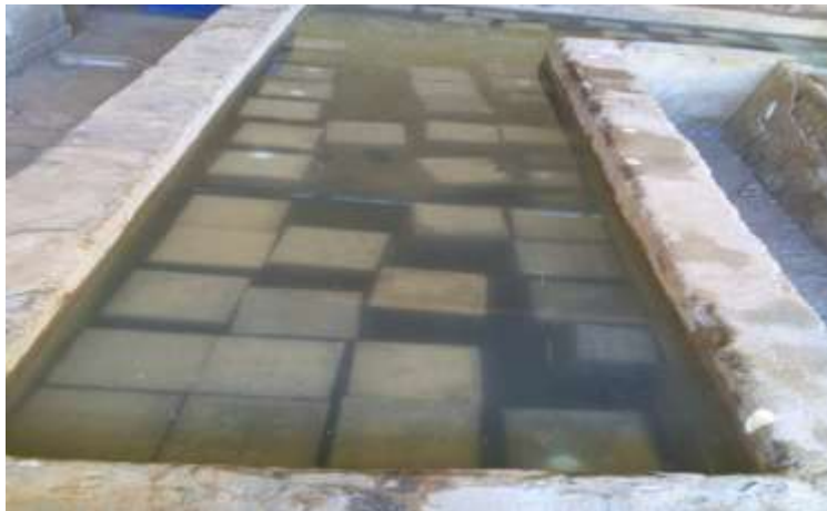
Figure (4.12): Cubes at curing basin
