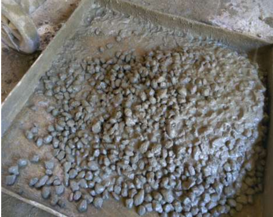
B1 concrete after mixing
