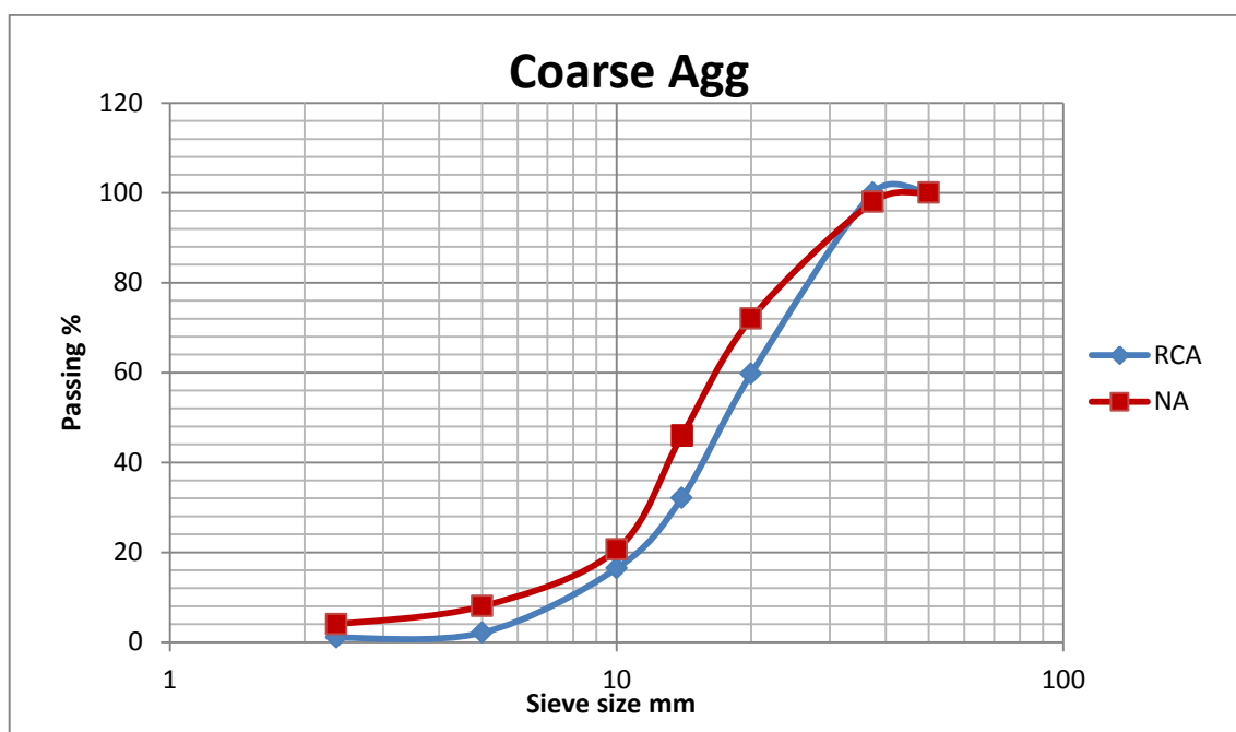
Figure (5.1) Logarithmic curve explain sieve analysis of coarse aggregate natural aggregate and RCA
