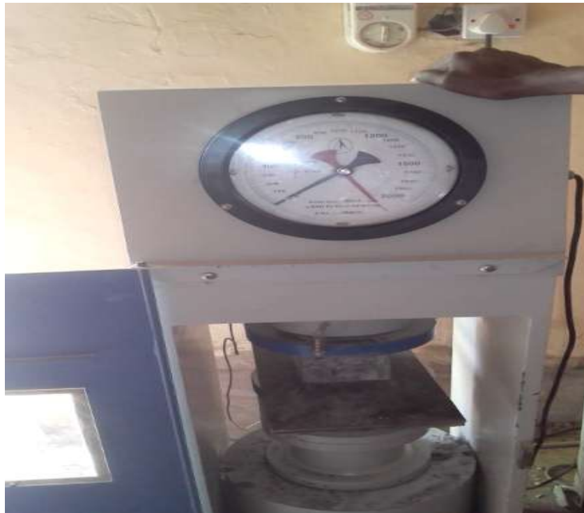
Figure (4.11): Compressive testing machine used in this study.
