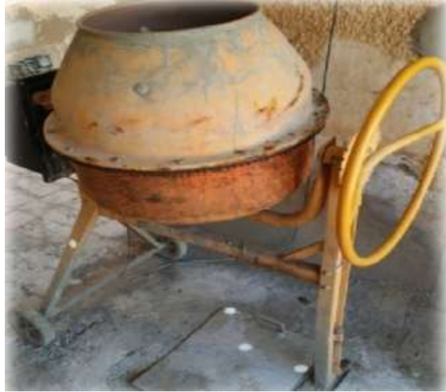
Figure (4.7): Drum mixer used for the mixing process
