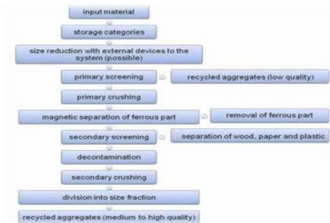
Figure (2.4): Scheme of a CDW treatment plant
