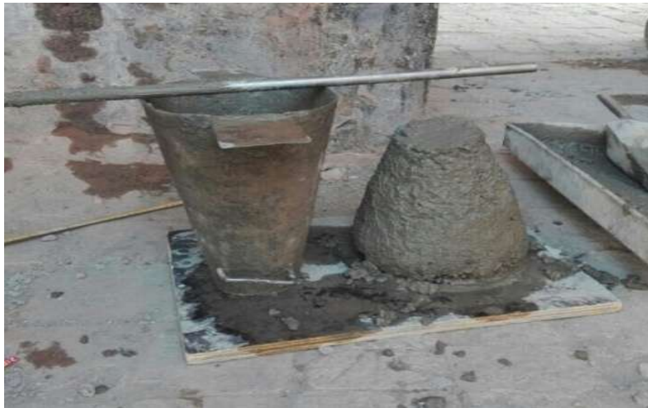
Figure (4.9): Slump test after mixing process
