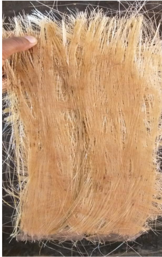
Fig (3.5): Quasi isotropic [0^0,90^0,45^0] sample.
