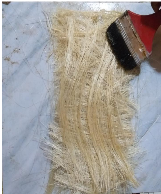
Fig (3.4): preparation of quasi isotropic [0^0,90^0,45^0] sample.
