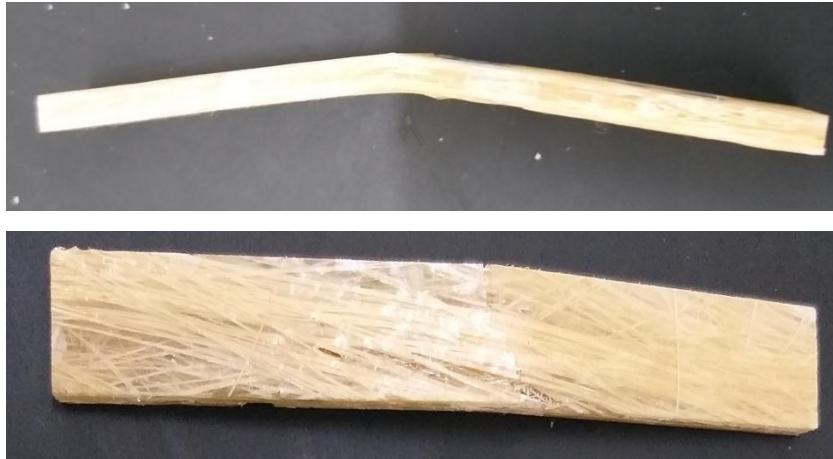
Fig (4.16): flexural specimens after failure.
